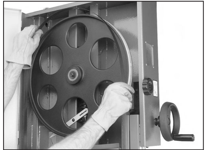
Figure 52. Placing blade on the wheels.
